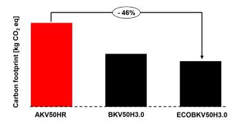
The use of a BKV50 type with Eco glass-fiber reinforcement could potentially have reduced the carbon footprint of the battery charger cover by 46 percent compared with a component made from polyamide 66 with conventional glass fibers in the same quantity.
