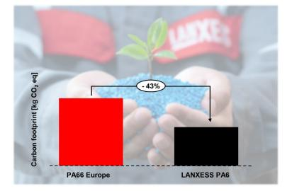
With 3.66 metric tons of  $CO_2$  equivalents emitted per metric ton of material produced, the carbon footprint of LANXESS' polyamide 6 base resin is much more than 40 percent lower than the current published European industry average for polyamide 66.
