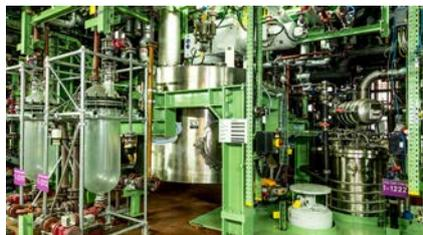
The paste bins in the Leverkusen production plant of Saltigo GmbH undocks the centrifuge and vertical mixer dryer as storage containers, thus reducing cycle times. Photo: Saltigo GmbH
