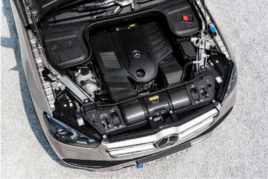
The Mercedes-Benz GLE SUV features a front-end support comprising two welded composite half-shells made from Tepex dynalite 104-RG600(3)/47%. The reinforcing glass-fiber rovings give the component a sporty look reminiscent of carbon fiber.
