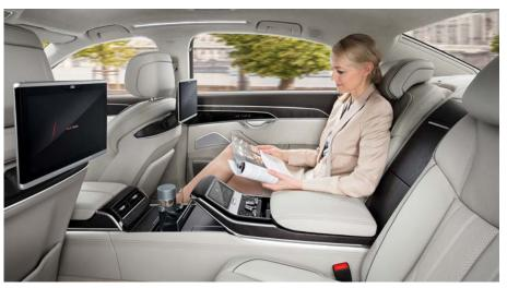
The Audi A8 is also offered with two electrically adjustable individual rear seats, the shells of which have been developed by Faurecia Automotive Seating and are manufactured using the hybrid molding process with Tepex dynalite 102-RG600(2)/47%. Photos: Audi AG
