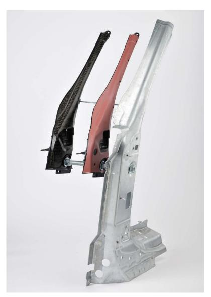
The 3D hybrid A-pillar extends upward from the vehicle rocker panel, accommodates the door hinges and holds the windshield in place at the side. Photo: LANXESS AG
