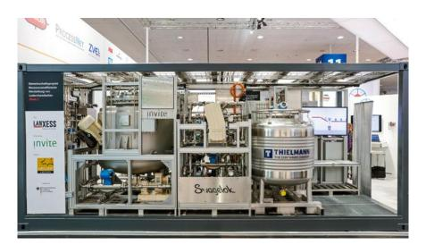
The modular plant for the "resource-efficient manufacturing of leather chemicals" is designed to produce retanning materials of the "X-Biomer" brand for the production of leather from shavings and biomass directly on site in tanneries. Photo: LANXESS AG
