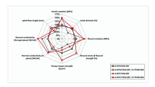
The properties of thermally conductive polyamide 6 compounds by way of comparison (freshly molded): Durethan BTC67ZH3.0EF and BTC77ZH3.0EF – the latest-generation Durethan TC products – are characterized by high impact resistance, elongation at break and flowability. Photo: LANXESS AG
