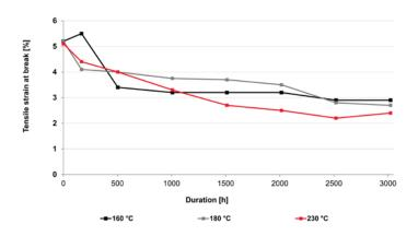
Strain at break of Durethan AKV320ZXTS2 after storage in hot air. The compound is almost completely resistant to brittleness under the influence of heat. Photo: LANXESS AG
