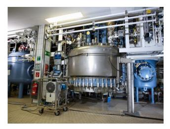
Cleaning of a nutsche filter in the Plant 3 of Saltigo GmbH in Leverkusen. Thanks to the 2.5 square meter filter area, approximately 800 kilograms of product can be filtered per operation. Photo: Saltigo GmbH
