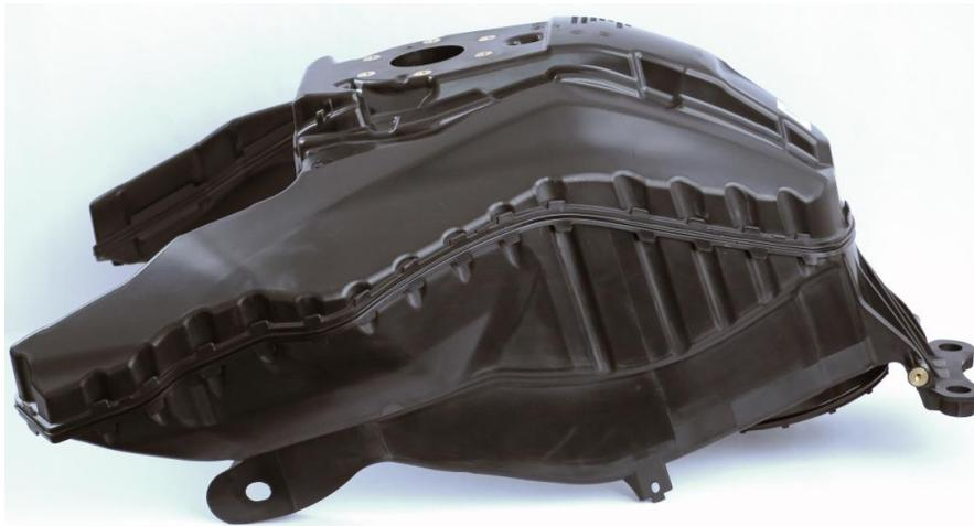
The motorcycle tanks of BMW Motorrad's models F 900 R and F 900 XR are made from Durethan BC550Z 900116 DUSXBL. The unreinforced and impact-modified polyamide 6 comfortably meets the stringent requirements of the United States Environmental Protection Agency (EPA) with regard to permeation. Furthermore, the complex geometries can be injection-molded cost-efficiently.
