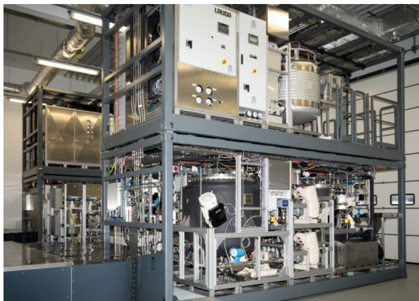
Modular plant for resource-efficient manufacture of leather chemicals. This plant allows tanneries to recycle shavings from leather production directly on-site and use these to produce X-Biomer retanning agents fully automatically. Photo: LANXESS AG
