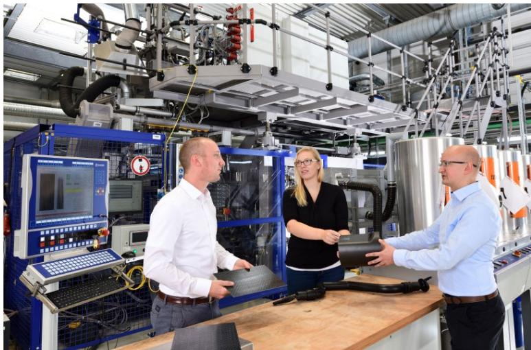
Engineering plastics experts Tilmann Sontag (left), Loreen Winkelhake and Arthur Rieb evaluate the quality of a hollow part reinforced with Tepex during blow molding at the Dormagen Technical Center of LANXESS's High Performance Materials business unit.
