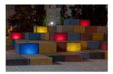
Twenty-four of the cubes that make up the "Urban Star" are made from translucent concrete, inside which special colored LED lights are embedded. During daylight hours, the sculpture's appearance is characterized by the cubes colored with LANXESS pigments. As twilight approaches, the translucent concrete becomes increasingly prominent. Photo: LANXESS AG
