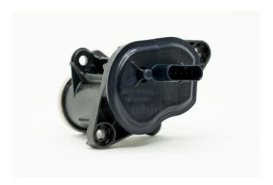
The cover of the actuator housing is made of black-colored laser-transparent Pocan B3233HRLT, while the laser-absorbing half of the housing is made of Pocan B3233HR.
