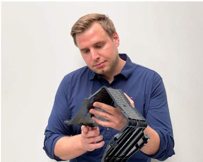
The bracket is designed to ensure that most of the forces are transferred from the points of application via the continuous glass fibers of the composite material.
