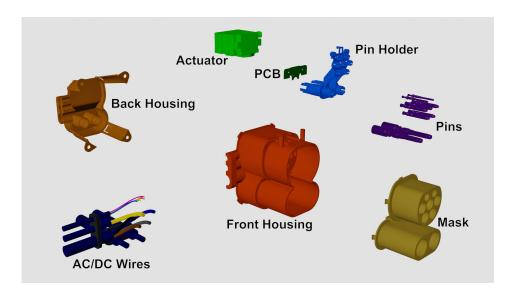
The charging inlet concept involves a modular design. Once the cables and contact pins have been placed in the holder and the PCB has been clipped in, all the components are put together with the aid of snap fits.
