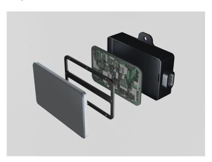
Structure of a radar sensor. For this application, LANXESS has materials that are characterized by good radar transparency, dimensional stability, good laser welding behavior or also excellent mechanical properties.
