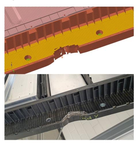
Crush test in the y direction: The results of the simulation match those of the physical component test very well.
