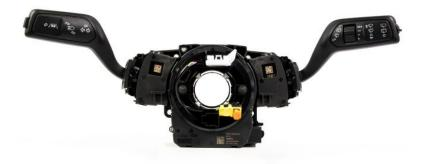
Substitution of polyamide 66 with polyamide 6 Durethan BKV30H3.0 in a steering column switch housing for different vehicle models from Ford. The component is manufactured using the foam injection molding process. The material switchover took place while the standard tool was in operation, supported by the LANXESS HiAnt engineering service. Photo: Kostal
