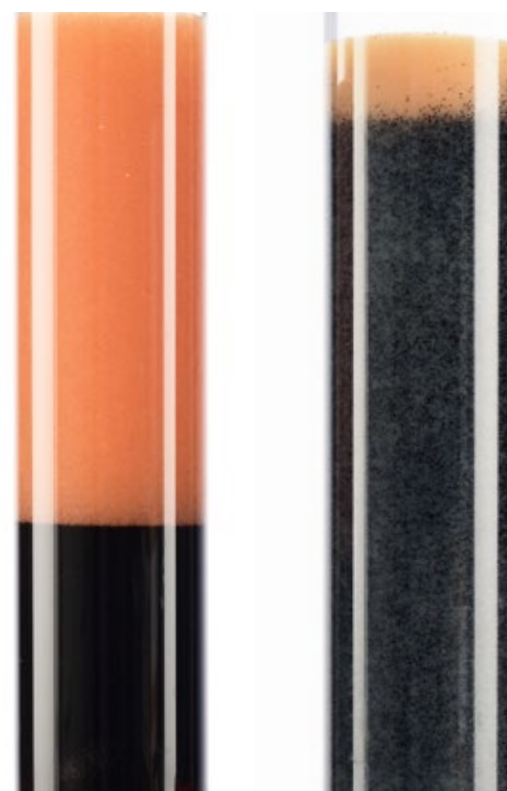
Fig. 13 Bad (imperfect) versus perfect pre-regeneration separation of SAC (dark) and SBA (light) of a mixed bed in a transparent column
