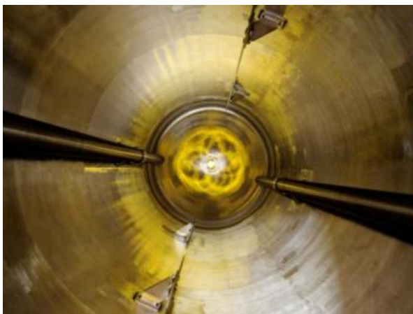
The view inside a stirrer vessel with a capacity of 12.5 cubic meters made from Hastelloy, an extremely corrosion-resistant nickel alloy. This material is used for the manufacture of agrochemical products, for example, which increasingly contain fluorine and exhibit corrosive characteristics. While stainless steel equipment would have been significantly cheaper, it would have offered only limited resistance when manufacturing these kinds of products. Photo: Saltigo GmbH
