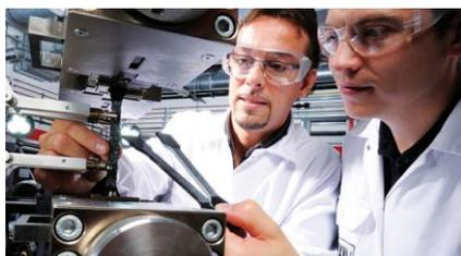
Marked specimens of the new, halogen-free, flame-retardant polyamide Durethan BKV45FN04 are clamped in a tensile testing machine. Photo: LANXESS AG
