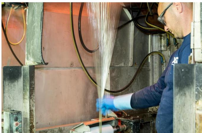
LANXESS glass fiber production at its Kallo site near Antwerp, Belgium. Photo: LANXESS AG
