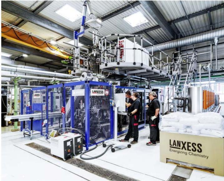
The new machine is a KBS20-SB extrusion blow-molding machine from Bonn-based Kautex Maschinenbau GmbH.
