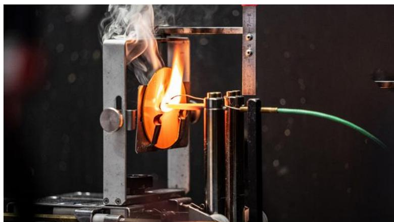
Among the new orange-colored polyamide compounds, Durethan BKV45FN04 stands out. The polyamide 6 exhibits high stiffness and strength and is very flame retardant. Photo: LANXESS AG
