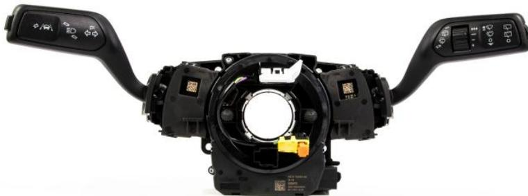
Substitution of polyamide 66 with polyamide 6 Durethan BKV30H3.0 in a steering column switch housing for different vehicle models from Ford. The component is manufactured using the foam injection molding process. The material switchover took place while the standard tool was in operation, supported by the LANXESS HiAnt engineering service. Photo: Kostal
