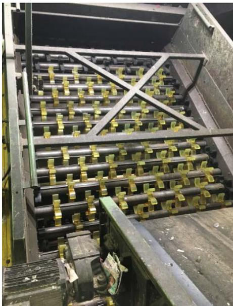
The PU star wheels based on Adiprene LF TDI are characterized by very high tear, abrasion and cut resistance and are resilient in humid and warm environments. Photo: LANXESS AG
