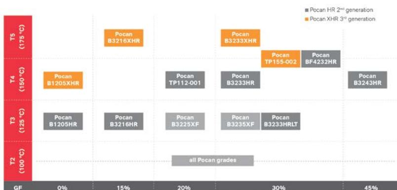
The Pocan XHR product variants achieve Class 4 or even Class 5, the two highest gradings in the USCAR tests. Photo: LANXESS AG
