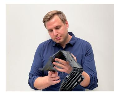
The bracket is designed to ensure that most of the forces are transferred from the points of application via the continuous glass fibers of the composite material. Photo: LANXESS
